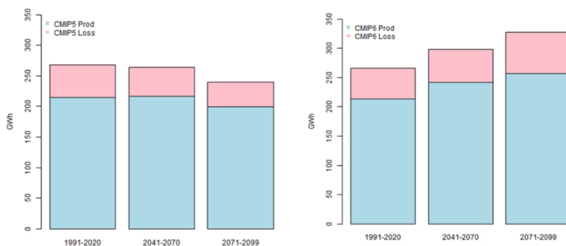
Figure 3.7. Annual mean hydropower production in light blue, and water loss (bypass and flood-loss) in light red the lower part of Krøderen subbasin: “less wet-scenario” RCP45 (left) and “warm-wet-scenario” SSP370 (right). Source: D4.2: Drammen (Hegdahl & Hisdal, 2026).
